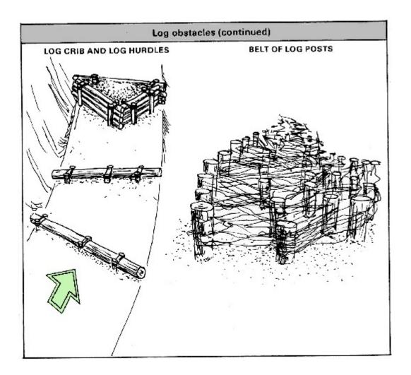
The effect of post type obstacles can be improved, and the obstacles made more difficult to breach, by weaving spirals of barbed wire among the posts. Exploding MOPMS into the obstacle after completion greatly increases its effectiveness. Conventional mines can also be used to make the obstacle more difficult to breach.
